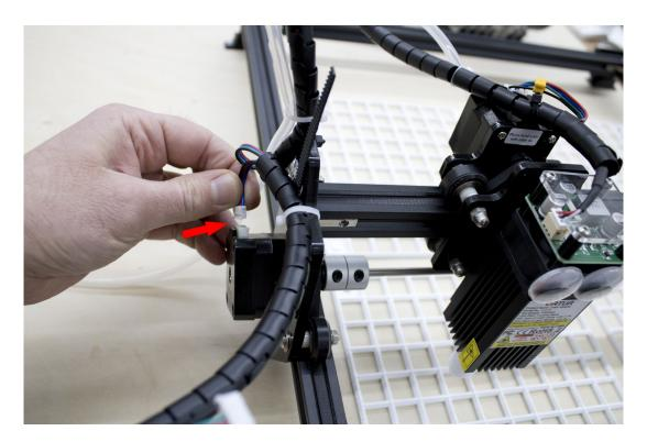
**3.** Carefully pull the cable out of the wire loom.
