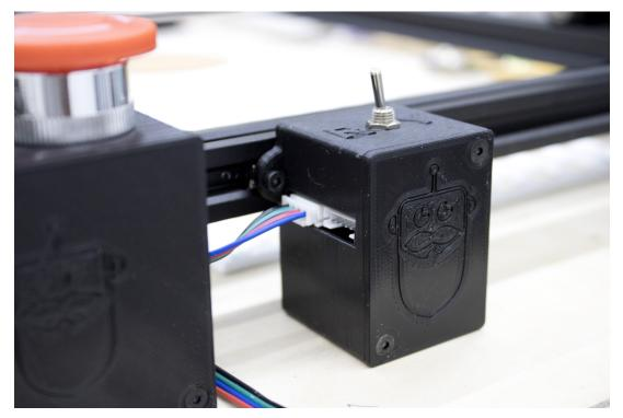
**8.** Plug the 6 pin end of the original Y Axis cable into the front port on the left side of the Y Axis Switcher.
