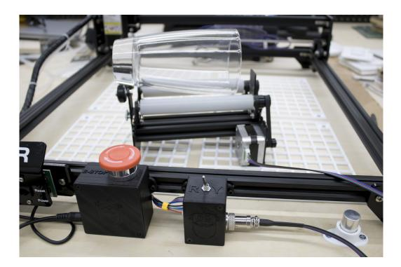
If you want to use the Ortur laser regularly, remove the rotary attachment and then flip the switch to the right.
