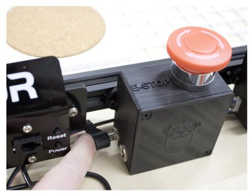
**5.** Plug the original power cable that came with your laser into the front port of the E-Stop. If you would like to cable manage the power cables, use the included zip tie.
