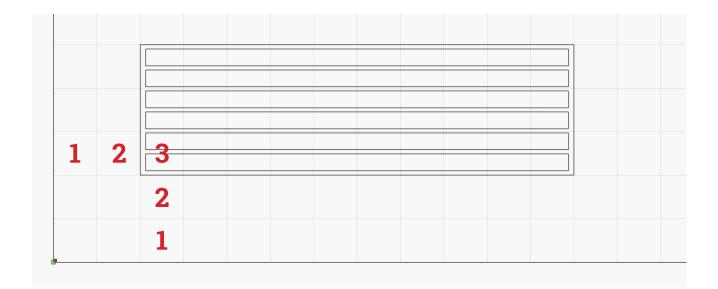
**2.** Now, you can place the pencil jig in the exact same location on the laser grid. Do a frame trace with the laser light on (Hold "Shift" while clicking the "Frame" button). Make sure the laser follows the outside of your jig.
