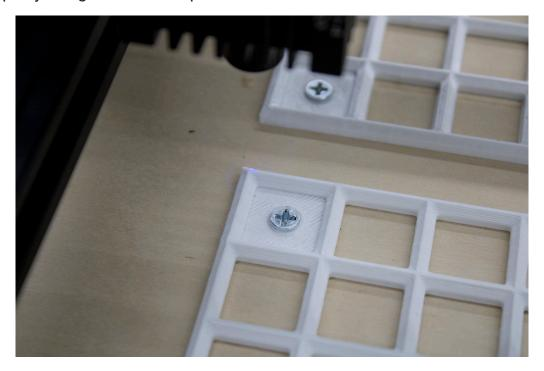
**6.** Once you have it square to the laser, move the laser 200mm (7.874in) to the right. It should ride along the top ridge of the Laser Grid to verify it is square. If it is off, make sure you are still square on the first two corners. If you are, check the squareness of your Grid and your laser chassis.
